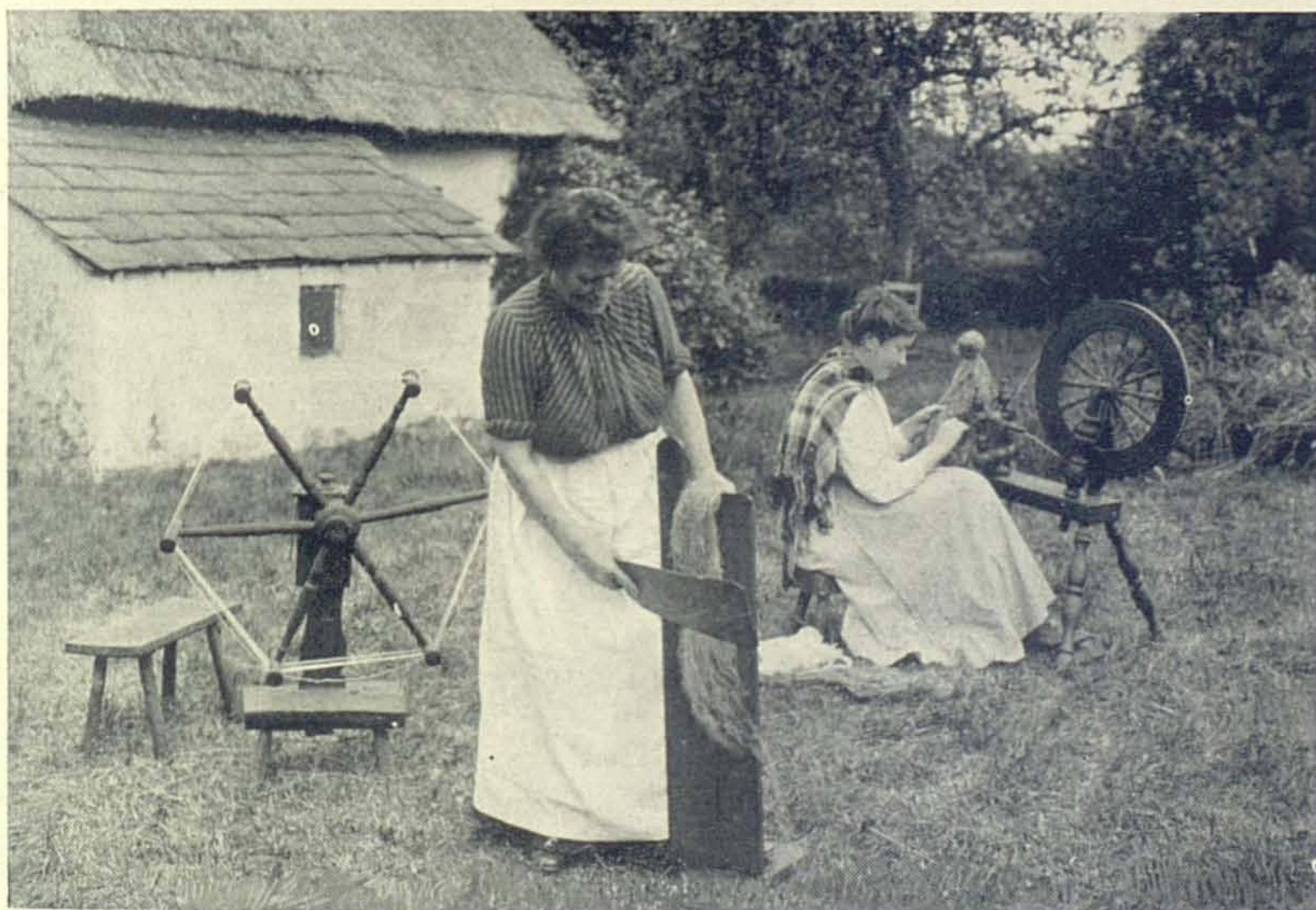
SCUTCHING STOCK, 'low Irish' SPINNING-WHEEL, and REEL, showing the kinds of implements used in the eighteenth century
